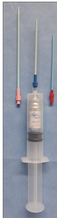
Figure 1: The syringe-actuated metered dose inhaler assembly
