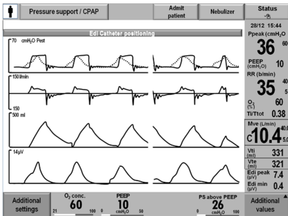
Figure 3: A drawing of the main screen of the SERVOi ventilator. This represents an adult patient in pressure support/CPAP mode. The top waveform is the pressure/time waveform (solid) and the Edi waveform (dashed line). The second waveform is flow/time, the third is volume/time and the fourth (bottom) is Edi/time. Note that the Edi signal from the diaphragm and the pressure waveform from the ventilator do not correspond. This is an example of patient-ventilator asynchrony (See text for further description).
