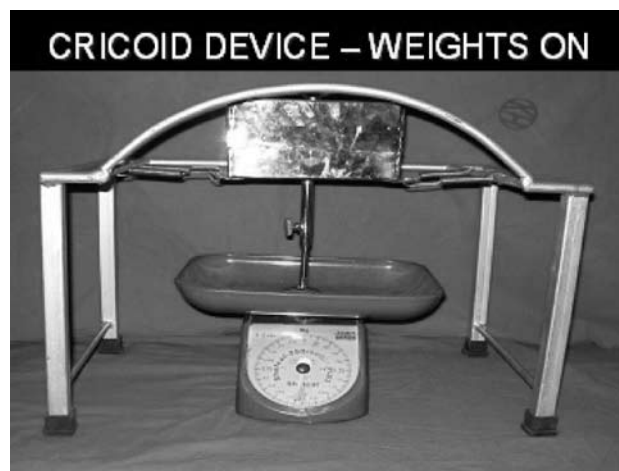
Figure 1: Cricoid device - checking the pressure and calibrating with weights concealed in the box attached to the stand by springs.
